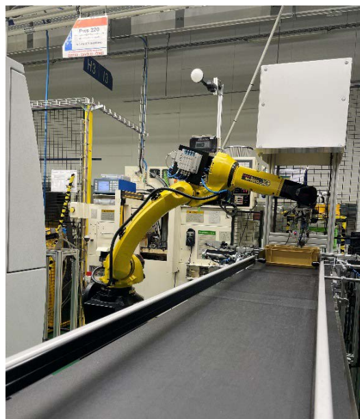
Robot FANUC M10iD/12 na lince P-EPS 2
